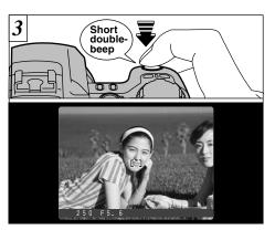
Press and hold the shutter button down halfway (AF/AE lock). The AF frame on the screen becomes smaller and the camera determines the shutter speed and aperture setting.
